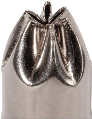
Figure 1: Ducta-bright 7a® withstands the extreme crimp of the Lehigh BPSIS Casing.
