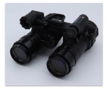
when changing positions to turn the IR illuminator on. The RNVG has IR signaling capability. As a safety feature, the switch knob must be pulled out to turn the IR illuminator on.
