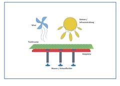
Hohenstein uses the WATson Heat Loss Tester measurement device to measure the cooling power of textiles..
