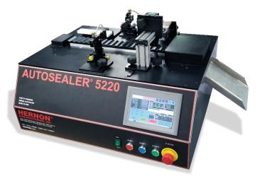
The new benchtop system is manually loaded by the operator and automatically aligns the cartridges into position for dispensing. After dispensing a wicking sealant onto the case-mouth and primer, the exposed sealant is cured in place using intense LED curing lights. Any non-exposed sealant cures anaerobically and the sealed ammunition comes off the machine ready to be handled, tested, packaged and shipped immediately.
