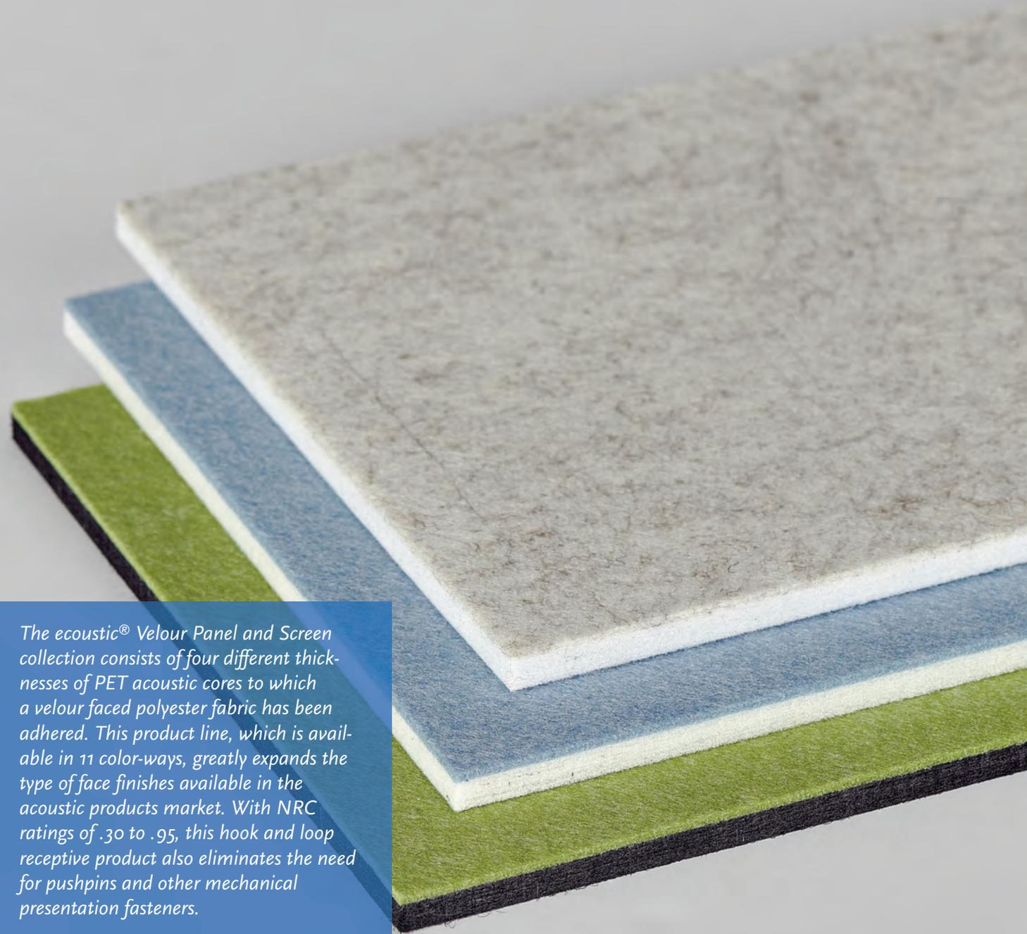
*The ecoustic® Velour Panel and Screen collection consists of four different thicknesses of PET acoustic cores to which a velour faced polyester fabric has been adhered. This product line, which is available in 11 color-ways, greatly expands the type of face finishes available in the acoustic products market. With NRC ratings of .30 to .95, this hook and loop receptive product also eliminates the need for pushpins and other mechanical presentation fasteners.*
