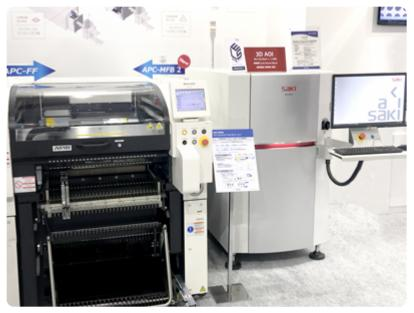
system to ensure mounting position accuracy. The system uses measurement results from SAKI's 3D AOI to analyze placement offset trends and optimize performance to improve SMT production-line process repeatability, accuracy, and yield. APC-MFB2 is an extension of Panasonic's APC-MFB and handles multiple package types such as small-outline and grid array packages.
