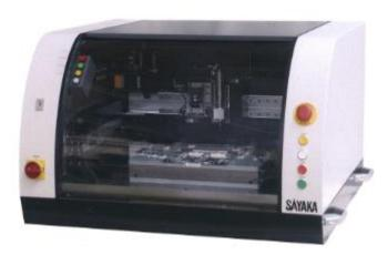
Seika has collaborated with Kawasaki Robotics Inc.'s engineering team to develop the Sayaka SAM-CT23NJ automated PCB depaneling system combined with the Kawasaki duAro dual-arm SCARA robot. With the new design, the robot performs the loading and unloading of PCBs onto the router.
