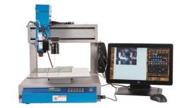
TS8100-100 Positive Displacement PC Pump is a continuously volumetric pump volumetric dispense designed based on Progressive Cavity (PC) technology. The pump can accurately dispense a wide range of fluids, from low viscosity coatings to high viscosity greases. The TS580R is a Smart PC Pump controller capable of controlling the Techcon TS8100 series PC Pump. With a universal power supply, it is a fully 'plug and play' system and can be used immediately, anywhere in the world.
